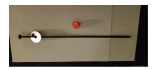
Figure 6 - A 12" monster panel screw and 1" Orange cap nail
